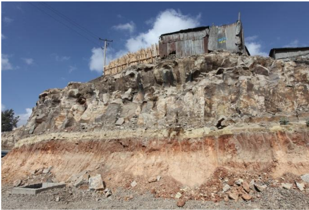
Engineering geology of the Addis Ababa Sheet (ignimbrite and paleo-soil at Debre Zeit road)
